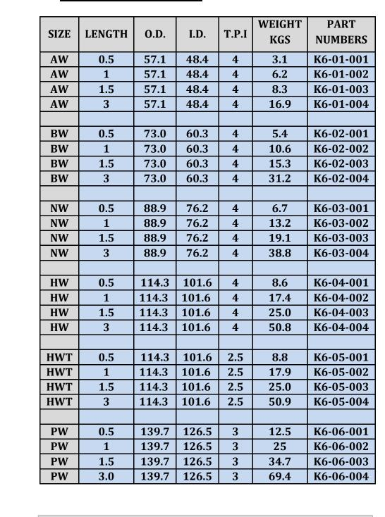
ALL AMKO CASINGS ARE MANUFACTURED FROM THE HIGHEST QUALITY RAW MATERIALS i.e. COLD DRAWN SEAMLESS TUBES OF GRADE SAE 1541 THAT ARE IMPORTED. THESE HAVE EXTREMELY HIGH MECHANICAL PROPERTIES AND STRAIGHTNESS BETTER THAN 1: 2000. ALL DRILL CASINGS ARE PARALLEL WALL.
